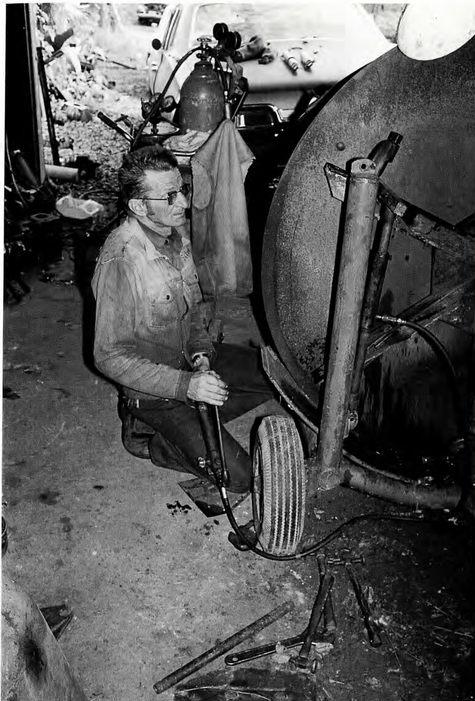
9 Willie pumping the Porta-Power to twist one arm of the blower.
