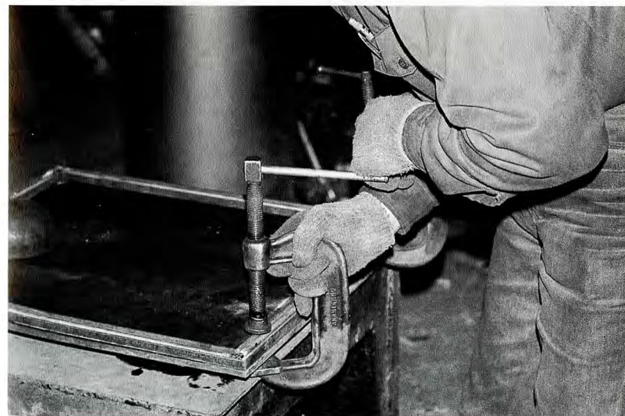
15 Clamping the mitered iron channel, part of the air seal, to the stove door.
