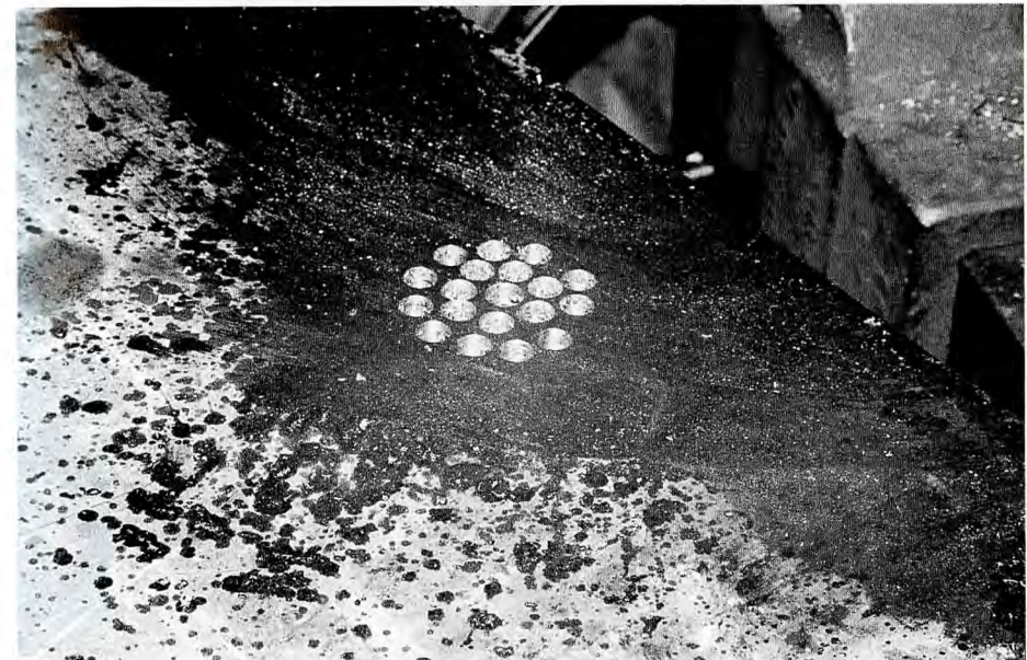
22 Damper holes. Willie will thread the center hole so the damper can be screwed in or out, regulating the amount of air blowing through the holes into the fire.
