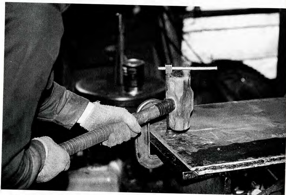
20 Using an eight-pounder to straighten the door.
