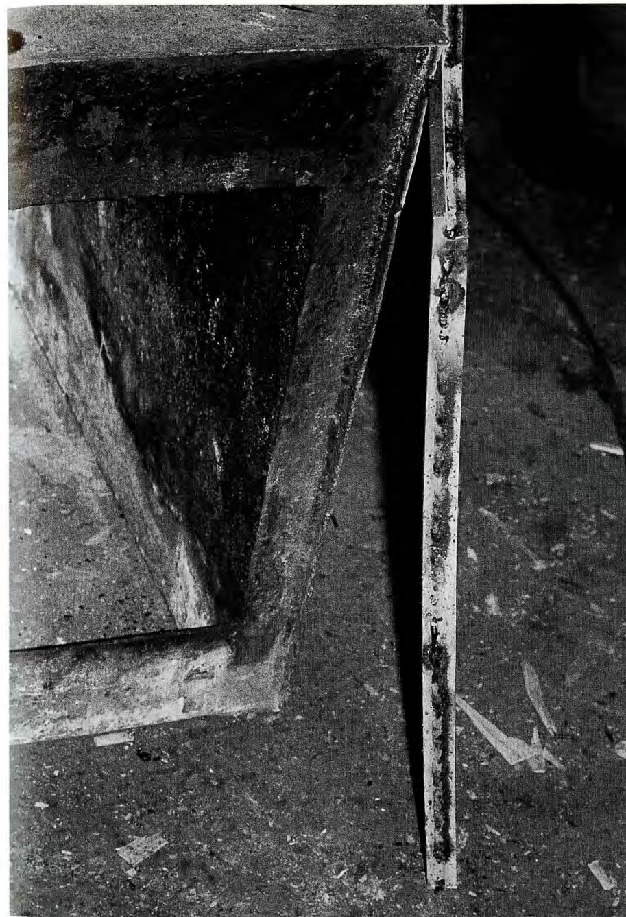
19 The warped door viewed from the edge. The channel is welded to the right side. The door leans up against the stove, here viewed from the front. Note the bow in the edge of the door facing the front.
