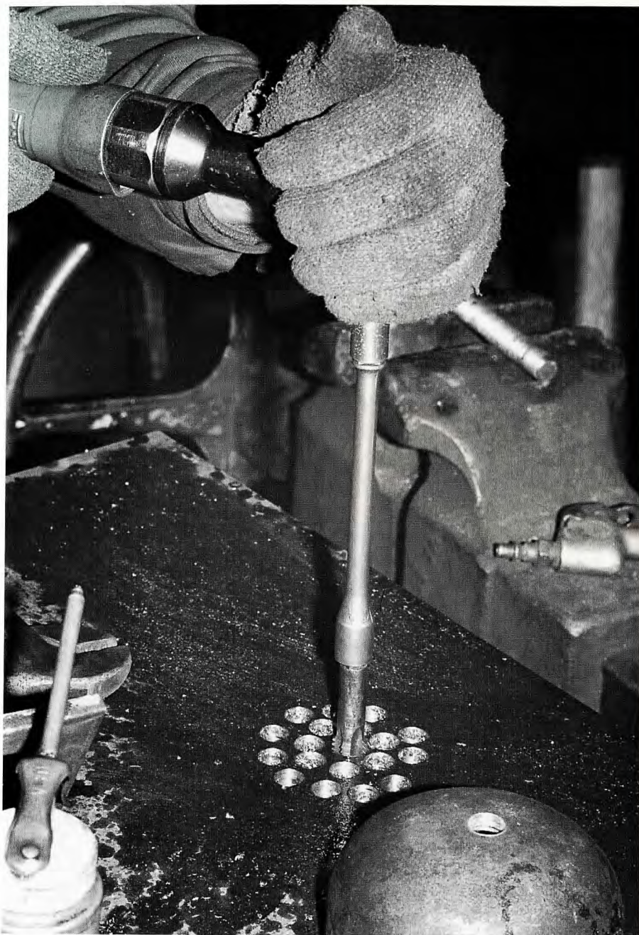
23 Willie cuts threads in the center hole with the air wrench. He has just threaded the hole in the damper, which is in the right foreground. He will weld bolt stock (cut from a long piece of threaded rod) into the damper, which can then be screwed into the door. With the damper turned in tight to the door, the fire is starved for air and burns more slowly. With the damper turned away from the door, the fire gets more oxygen and burns hotter.
