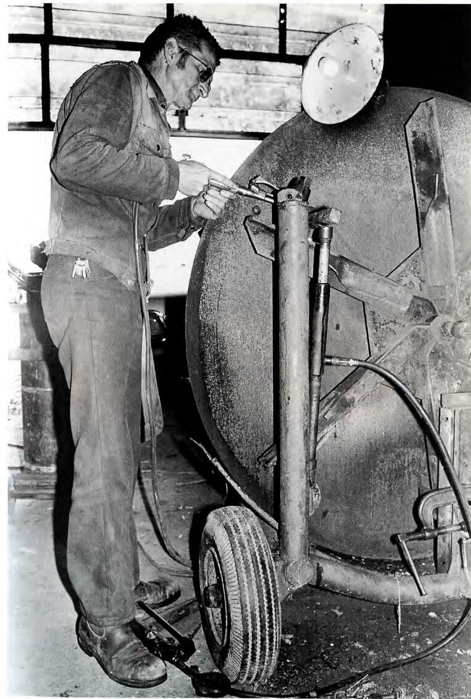
10 Willie heats the arm of the blower with an acetylene torch so it will "take" the twist.
