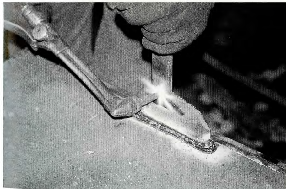
31 Willie heats the handle and bends it so that pushing it into the jaw will draw the door tighter to the stove.
