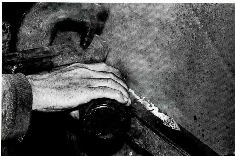
12 Pouring water on the metal to make a water bend.
