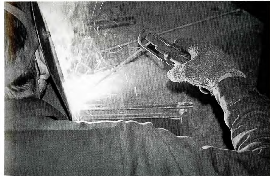
18 Willie welds the door. The reinforcing-rod seal sitting on top of the stove will be welded onto the front of the stove so that the channel closes over it.
