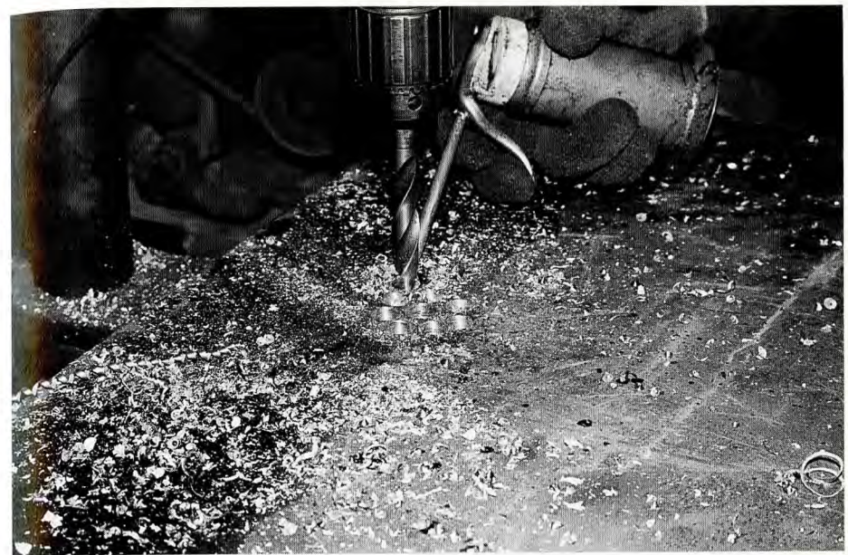
21 Willie drills air holes in the door.
